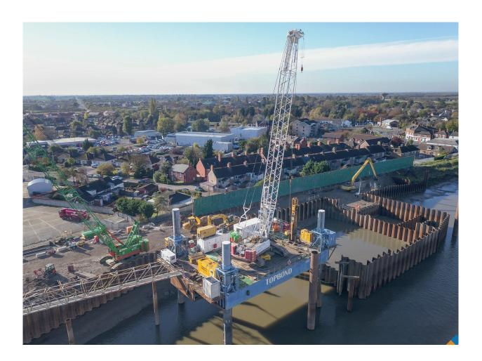
**TOPJACK** is a modular **Jack Up** barge with 250 tonne lift capability complete with 36m legs. Capable for supporting a wide range of disciplines including port construction, safe investigation and piling operations.
